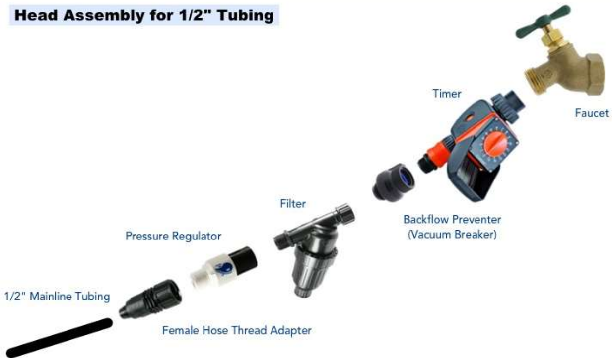
Fig.3 assembling of drip irrigation
